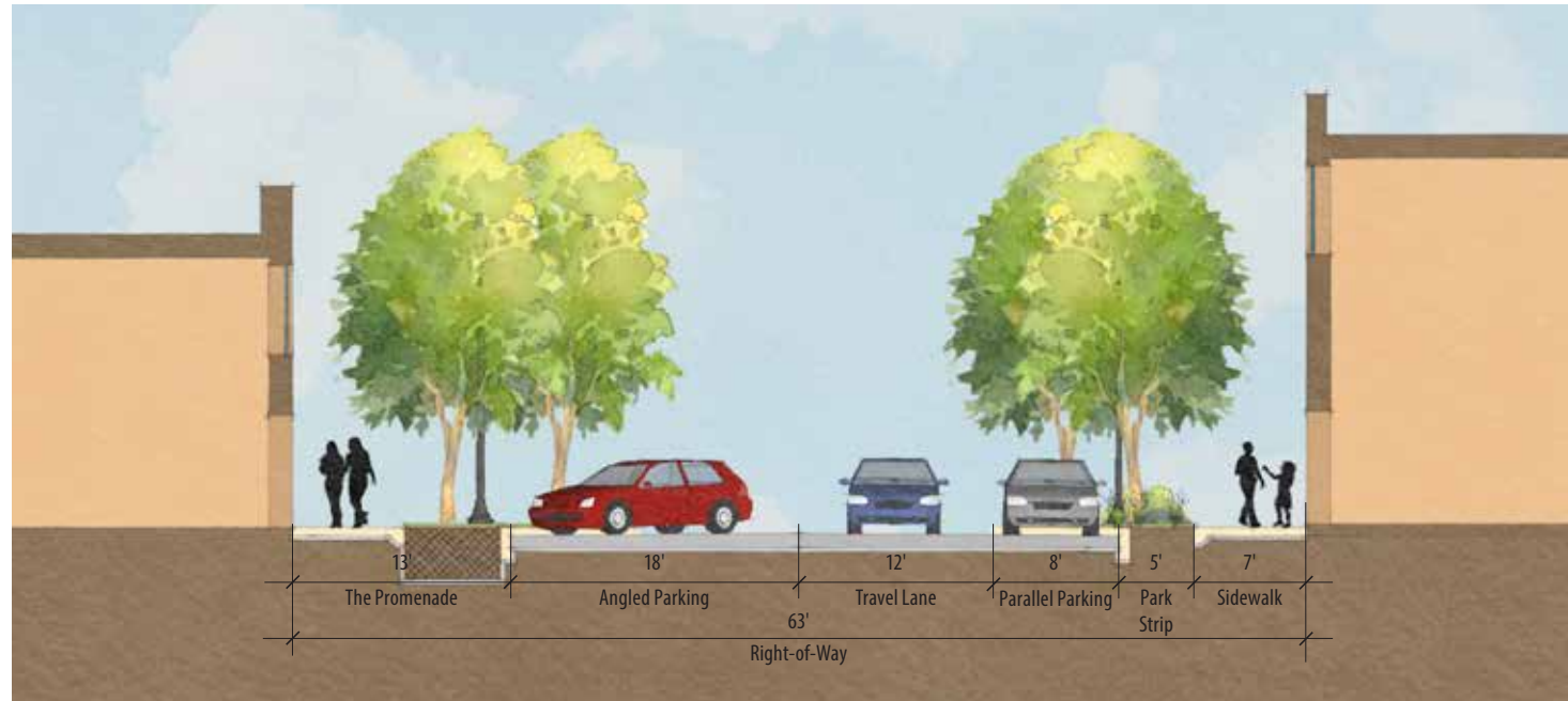
Fig. 29 41½ AVENUE PROPOSED STREET SECTION OPTION 1 One side of diagonal parking and one side of parallel parking take advantage of the current paving area and provide plenty of street parking, while the widened sidewalks help achieve the desired pedestrian-friendly character.
