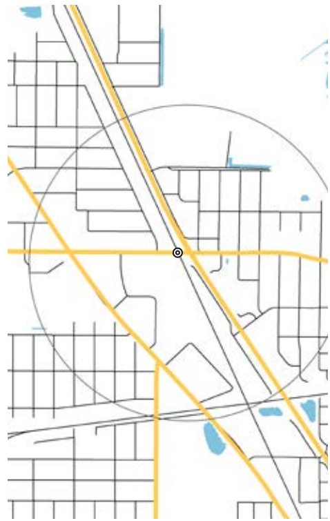
Fig. 9 LOCAL STREET PATTERNS The station area is characterized by a grid of local streets that is interrupted by West Broadway Avenue and two freight rail corridors. These major infrastructure elements have limited crossing points, funneling traffic onto a few crucial arterial streets, such as Bass Lake Road.
