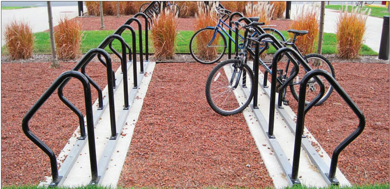
**Recommended — D shaped or swerve racks:** Can stand alone for curbside use or multiple parallel racks can be installed for high density uses in bike corrals. *Credit: Dero Bike Racks*
