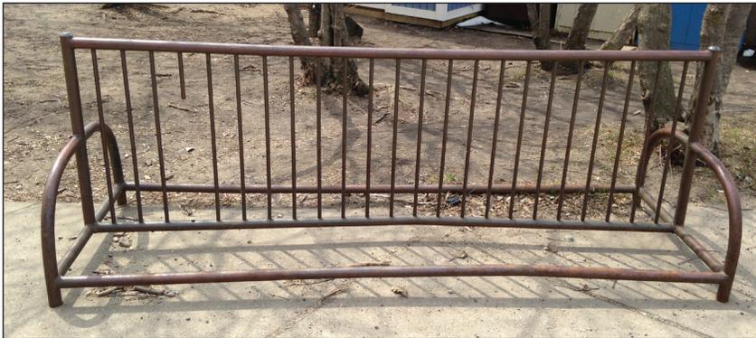
**Discouraged — Comb or schoolyard:** May damage front wheel and does not allow users to lock both frame and wheel to the rack.
