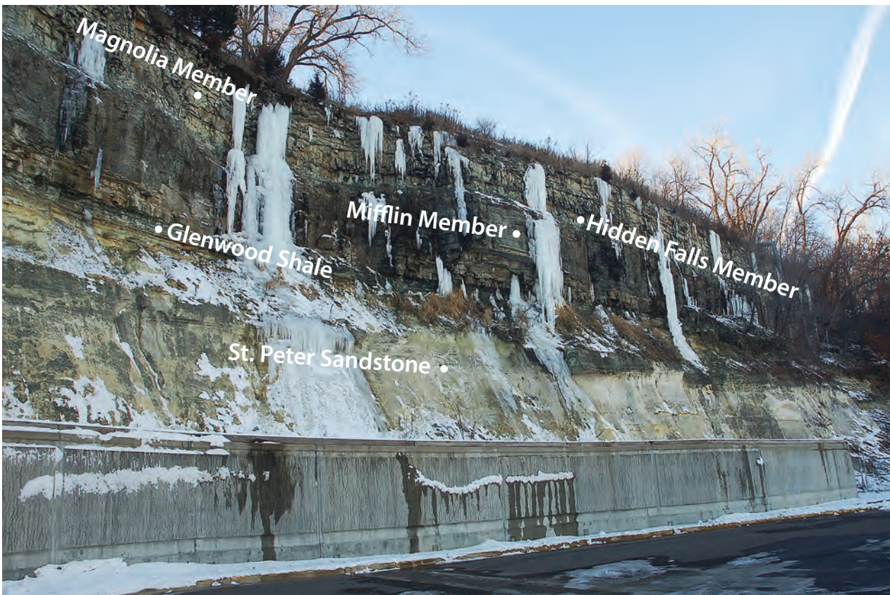
Figure 7.3 — Bedrock Sequence The Magnolia Member is 7–10' thick and has a blocky appearance. The Hidden Falls Member is 4–6' thick and has curvilinear fractures. The lowermost Mifflin Member is 11–13' thick and breaks off in large, tabular slabs. Springs emanate predominantly from Magnolia/Hidden Falls contact (48%) and Hidden Falls/ Mifflin contact (25%). Seeps along bedrock layers exposed above the Ford Dam can be identified by ice. ( Runkel et al., 2015 )
