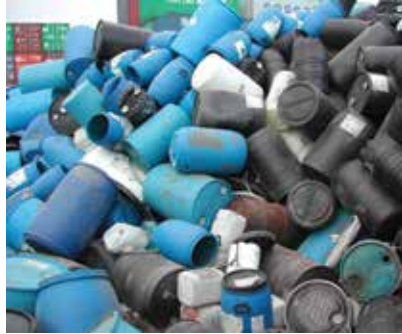
These containers are NOT being managed properly. They should be managed according to RCRA standards.
