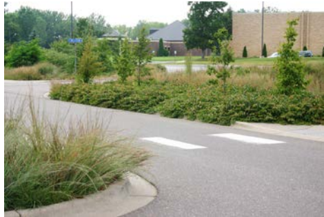
Design safe walkways and parking lots; consider sight distances and mature plant heights along roadways.
